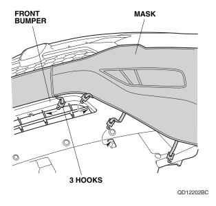
5. Attach one hook to the hole on the front bumper. Repeat on the right side.
